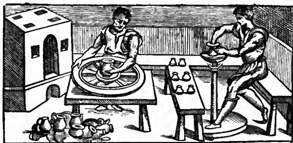
FIG. 5.—Two forms of Italian potter's wheels, about 1540.
