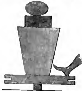
FIG. 2.—Potter's wheel of the time of the Ptolemies, moved by the foot (from a wall-relief at Philae). Compare fig. 5, the wheel on the right.
